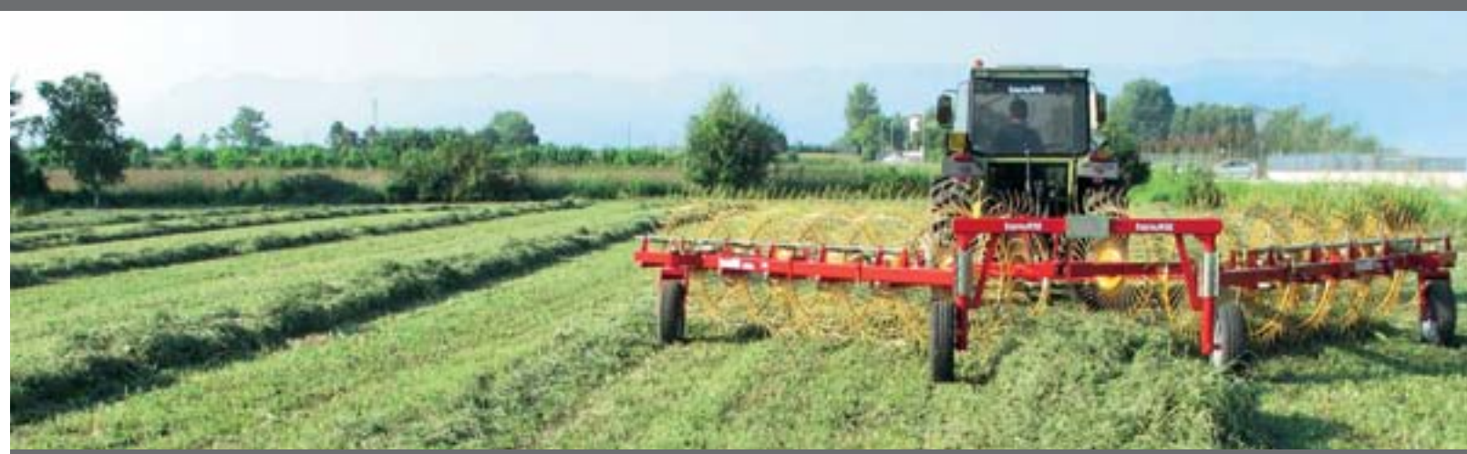
Tandem wheel kit with tires with special tread for a better stability on inclines or in hilly areas (optional).
