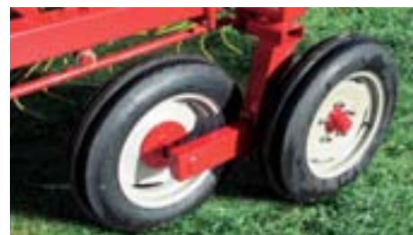
Tandem wheel kit with tires with special tread for a better stability on inclines or in hilly areas (optional).
