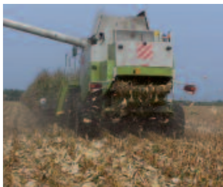
Corn harvesting with built-in stalk chopper.
